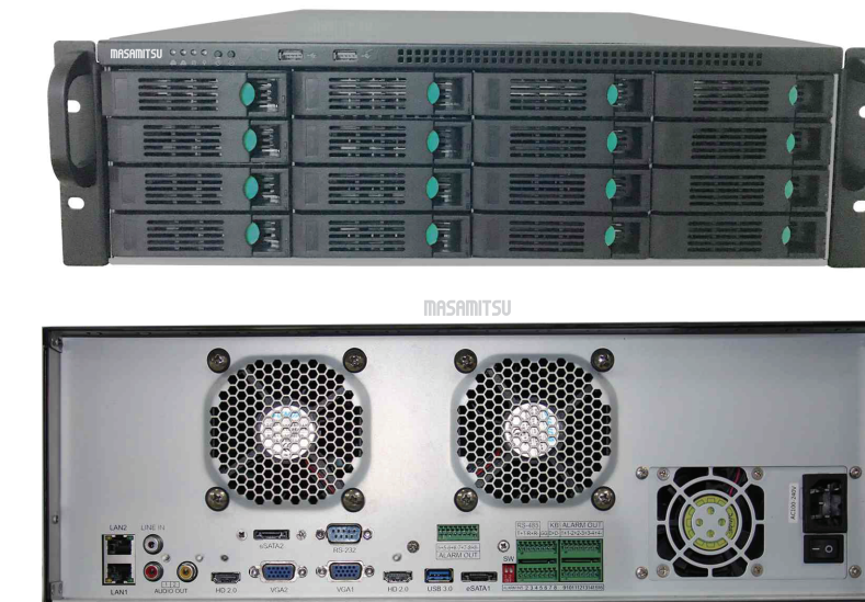
16HDD 4.0U CASE L437*W483*H143 mm
